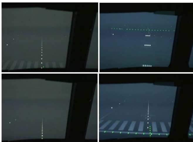
Figure 8. OTS CAT II approach: normal (left) versus -10m bias (right) at 100ft / 50ft / 20ft
