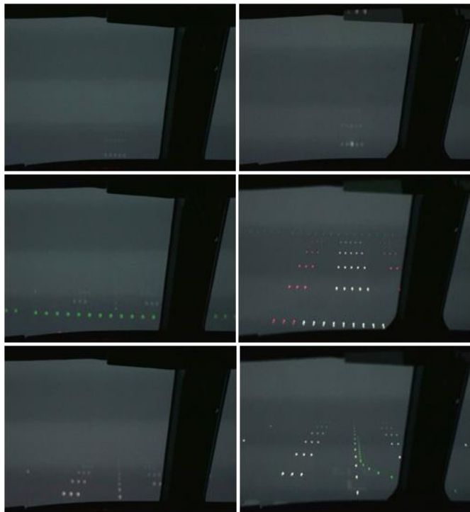
Figure 7. CAT II approach: normal (left) versus -10m bias (right) at 100ft / 50ft / 20ft
