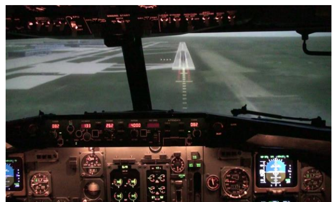
Figure 21. Outside View of Short Final with 4° glide and 4 white lights on PAPI
