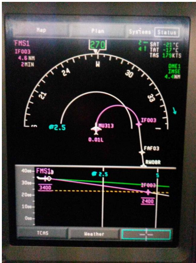
Figure 2. Navigation Display with Radius-To-Fix Procedure and Vertical Path
